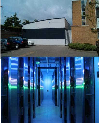
It's a High-Density data centre (up to 24kW per cabinet) Tier-3, lights out facility 365 Free-Cooling Efficient Flywheel UPS (98% at 100% load and still 96% at 40% load) Annualised PUE of 1.05 100% Renewable Energy Rain Water recapture Energy Efficient Transformer No Waste in the Construction
